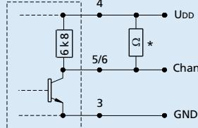
\* An additional external pull-up resistor can be added to improve the rise time. Caution: Iour max. 5 mA must not be exceeded!
